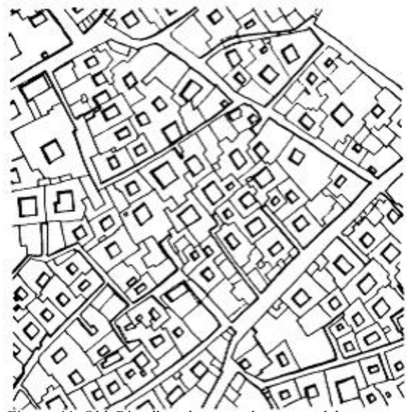
Figure 11 Old Riyadh, where mud courtyard houses are similar in height (one story), none of which blocks the air from reaching the others.
